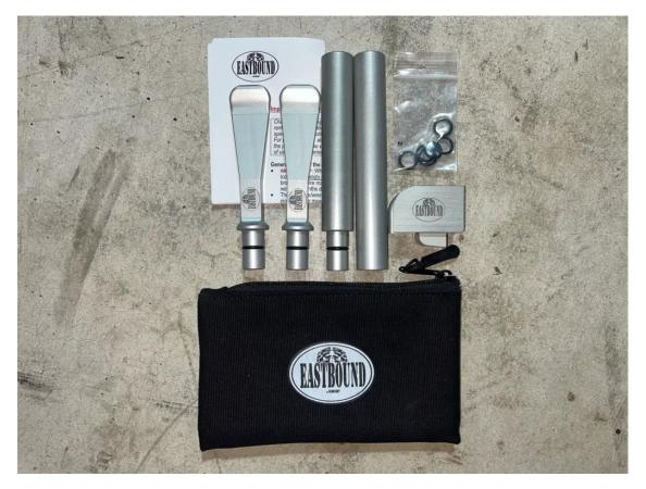
Based in The Netherlands, Eastbound is known for its compact, carry-along tool kits for servicing motorcycle wheels and repairing tires. The Eastbound Tyre Repair Kit consists of universal tire spoons and a unique fulcrum for bead-breaking. The Wheel Service Kit is a model-specific set of tools for removing axles and associated pinch bolts.
