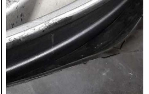
Step 8; The bead breaker will open and push the tyre and rim apart. The tyre must be pushed over the safety hump inside the rim. If the tyre is not pushed off the first time, repeat the action two inch to the left or right.
