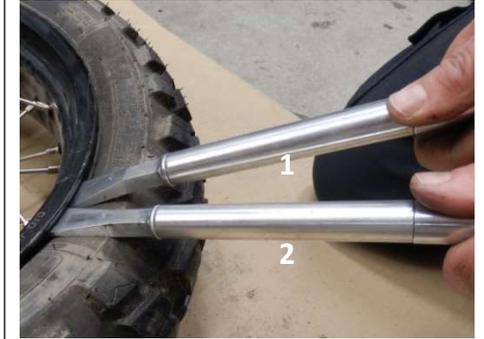
Step 4; Push spoon 2 as deep as possible while keeping downward pressure on spoon 1. The tip of spoon 2 should catch behind the tyre bead. You can feel it when it does.
