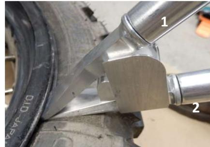
Step 6; Place spoon 1 in the fulcrum with the tip pointing up. Push spoon 1 carefully between the rim and the tyre. Make sure that spoon 2 stays in place. Be careful not to push spoon 1 over the rim. This could cause scratches. If spoon 1 does not slide easily between rim and spoon 2, wiggle spoon 2 up and down to create space. See (\*)
