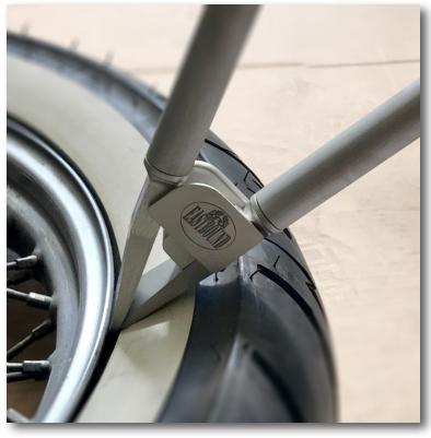
The great thing with the Eastbound Tyre-Pro is that the design meant that the rim was not damaged, even without the use of rim protectors - we removed the protectors after a few seconds! (*They don't come with the kit*)
